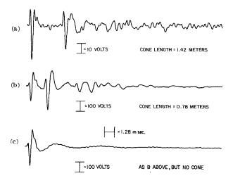
g. 1. Ensemble sum of 50 25.6-ms epochs from output of sound meter. (a) Sound meter acoustically coupled to absorber via a 1.42-m paper cone. (b) Same as (a), except transmission distance was reduced to 0.78 m. (c) Same as (b), except the cone was removed which tended to acoustically decouple the sound meter from the absorber. Fig.
